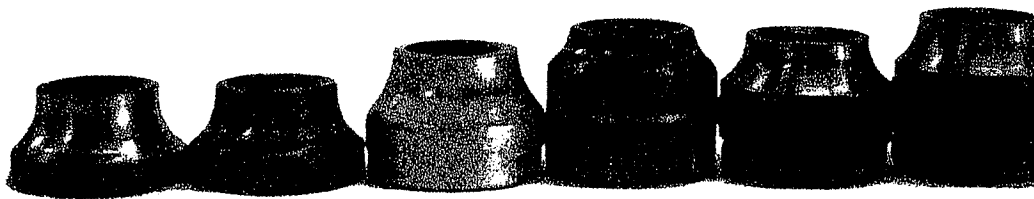
Fig. 12 - An assortment of cones for a cup and cone hub bearing assembly. Note the wide variation in dimensions.
