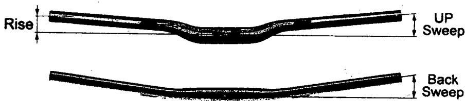
Fig. 11 - Upright handlebars. Top: a riser handlebar viewed from the front. Bottom: the same bar viewed from above, showing back sweep.
